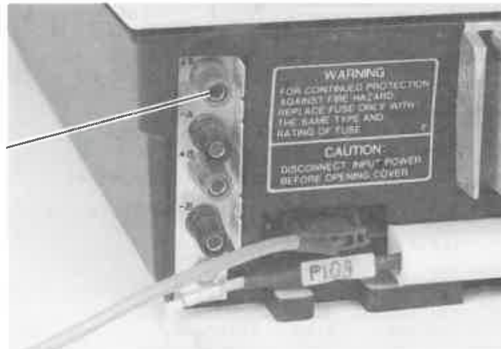
Figure 1.4 Detector Input Connections (banana jacks) to the SP4200
